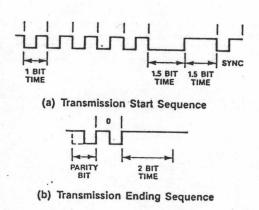
Figure 3.1 Transmission Start and Ending Sequence
