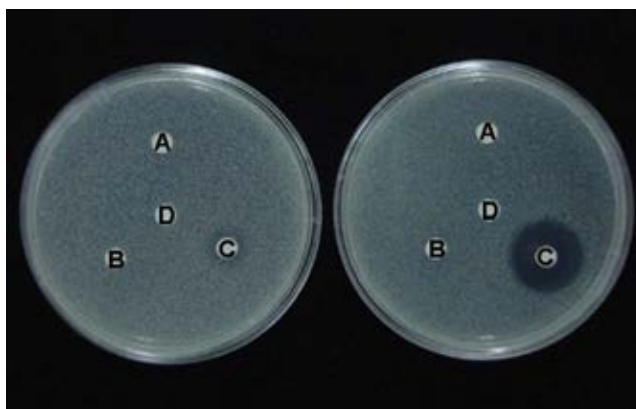
Figure 30 Disk diffusion assay determining synergistic activity with ketoconazole against C. albicans of the isolated secondary metabolites (256 \mu\text{g} per disk, each) from A. alternata Tche-153: the left SDA plate without ketoconazole, the right SDA plate with a subinhibitory concentration of ketoconazole (0.125 \mu\text{g/ml} ), A = altenuic acid [53], B = 2,5 dimethyl-7-hydroxychromone [50], C = altenusin [43], and D = dimethylsulfoxide (control).
