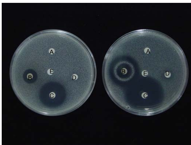
Figure 29 Disk diffusion assay determining synergistic activity with ketoconazole against C. albicans of the isolated secondary metabolites (256 \mu\text{g} per disk, each) from Nodulisporium sp. Aann-134: the left SDA plate without ketoconazole, the right SDA plate with a subinhibitory concentration of ketoconazole (0.125 \mu\text{g/ml} ), A = 1,8-dimethoxy naphthalene [18], B = 1,8-dihydroxynaphthalene [63], C = 1'-(2,6-dihydroxyphenyl)butanone [20], D = nulisporin G [62] and E = dimethylsulfoxide (control).
