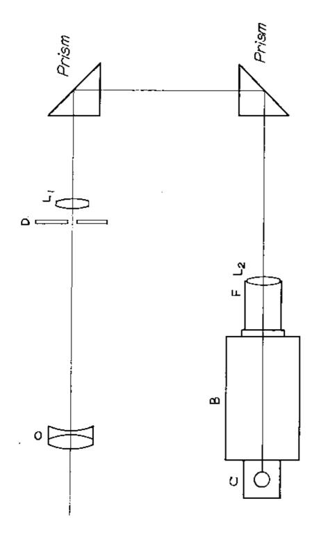
THE C.S.I.R.O. CHROMOSPHERIC TELESCOPE WITH BAND TUNABLE BIREFRINGENT FILTER AND CINECAMERA Figure 2-1
