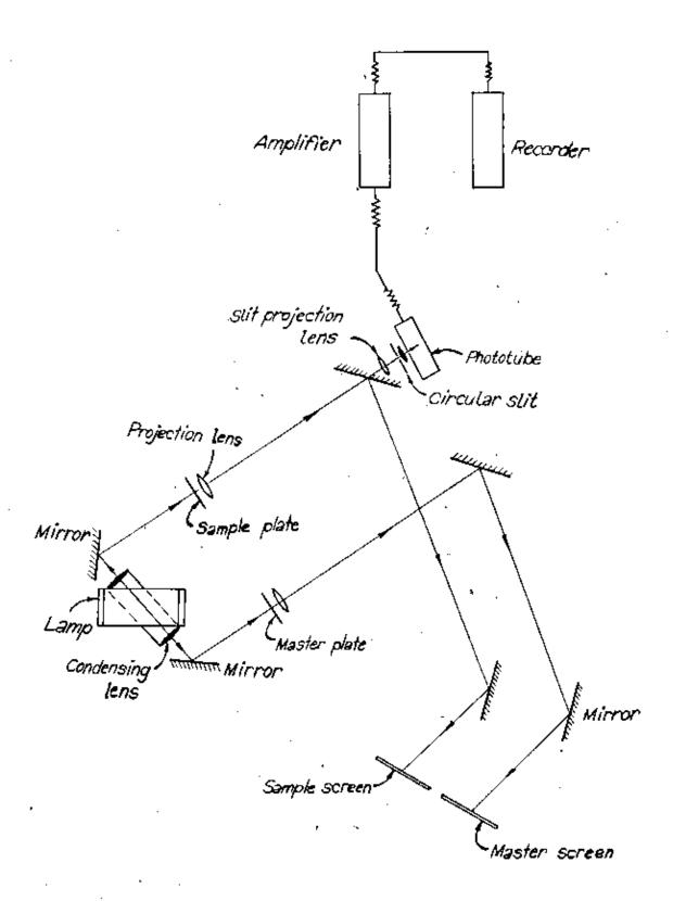
Figure 2-3 OPTICAL SYSTEM OF THE SPECTROSCANNER
