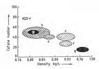
Figure 1.1 Typical properties of gas-oil components
