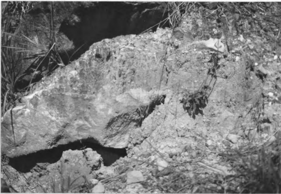
Figure 2.11 The fresh soil movement in the colluvial slope.
