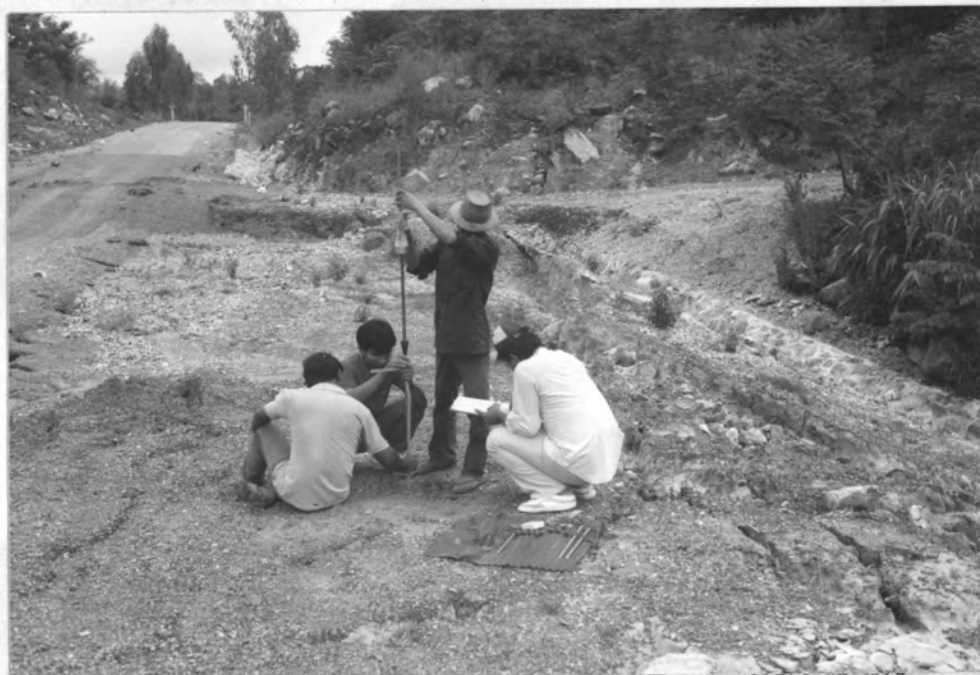
Figure 6.4 Examination of soil layers by simple sounding penetration test in the landslide area ( August 1985).
