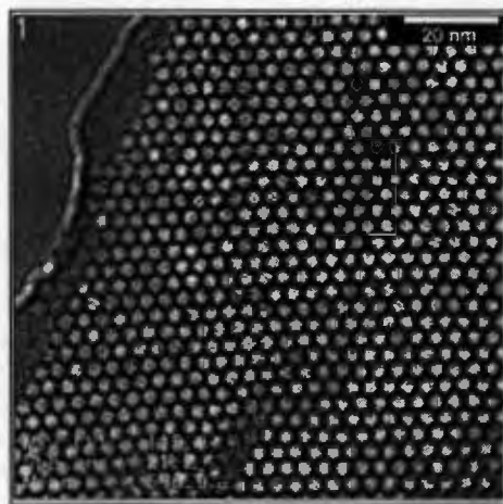
Figure 2.10 Transmission electron micrograph of MCM-41. [44]
