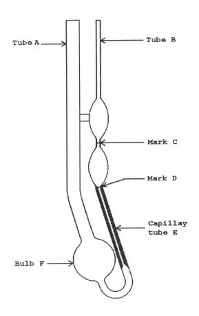
Figure 3.3 Cannon-Fenske Routine viscometer
