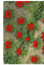
(c) The result of third erosion from Figure 73 (b) is on the left and the result of identification of individual oil palm is on the right
