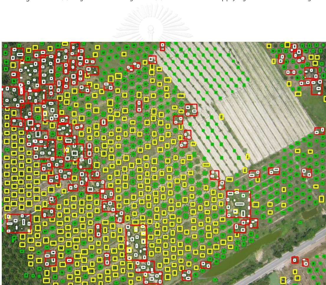
Figure 122 The result of multi-scale clustering from Figure 121 (b) including 428 small trees, 414 big trees, and 91 tree stands consist of 314 individual oil palms
