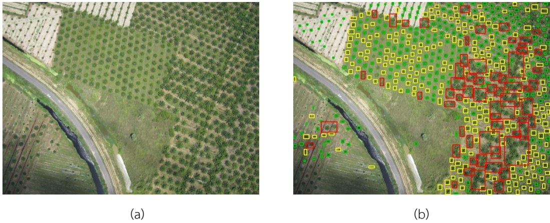
Figure 123 (a) original aerial image and (b) the result from applying K-means clustering
