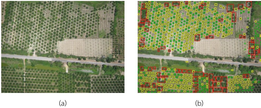
Figure 133 (a) original aerial image and (b) the result from applying K-means clustering
