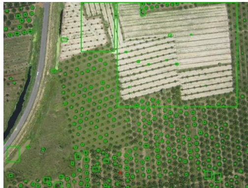
Figure 88 The far-distance aerial image with median-size oil palm smaller than the threshold size
