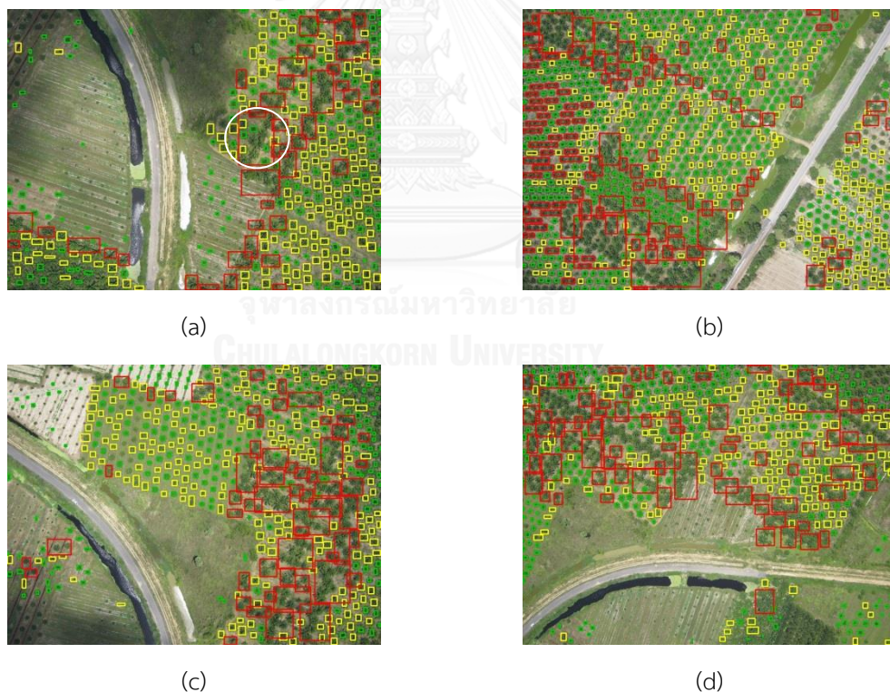
Figure 71 The results from applying K-means clustering to separate oil palms into three clusters of small trees (green), big trees (yellow), and tree stands (red)
