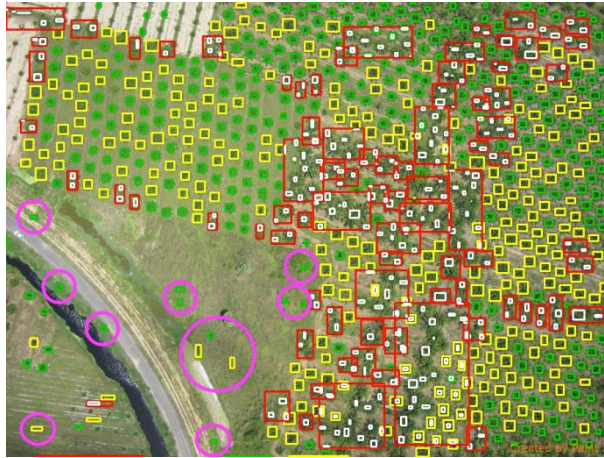
Figure 112 An example of false detection from K-means clustering
