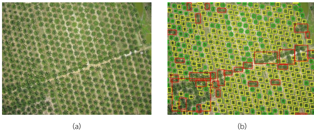
Figure 153 (a) original aerial image and (b) the result from applying K-means clustering
