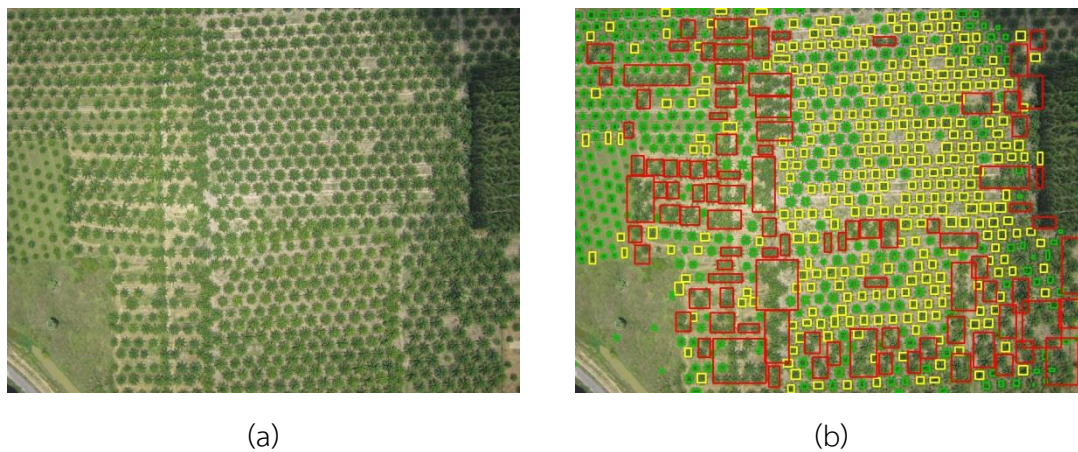
Figure 149 (a) original aerial image and (b) the result from applying K-means clustering
