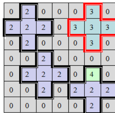
Figure 63 The process of first scanning is repeated until all the first pixels are scanned
