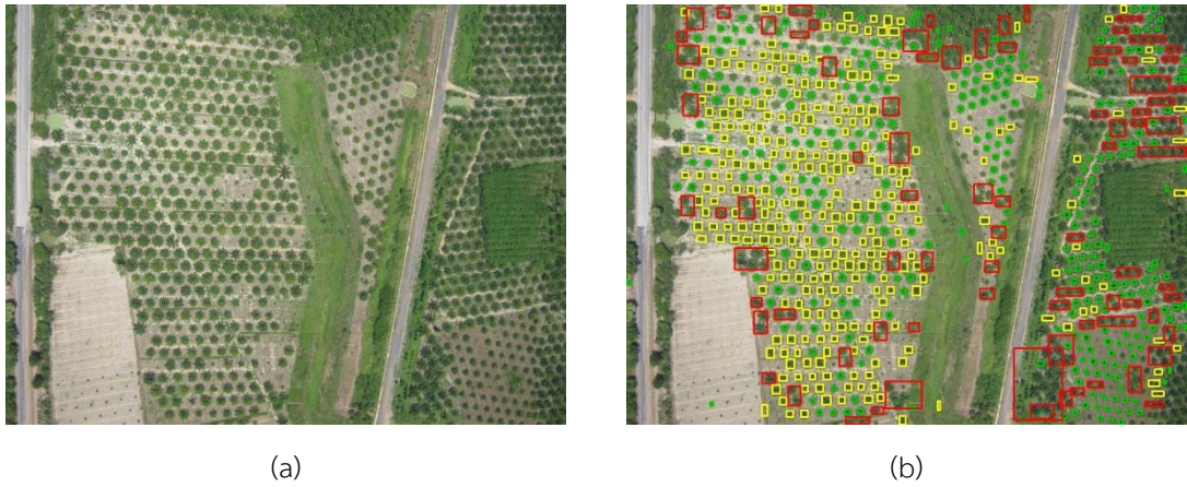
Figure 135 (a) original aerial image and (b) the result from applying K-means clustering
