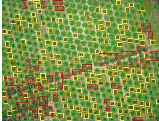
Figure 74 K-means clustering result of an aerial image
