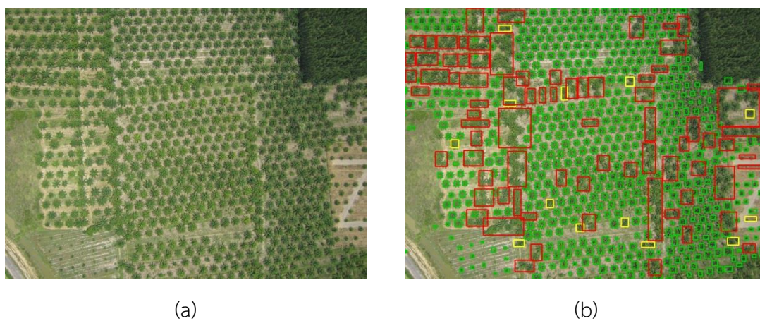
Figure 145 (a) original aerial image and (b) the result from applying K-means clustering
