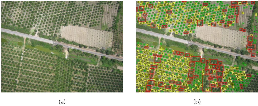
Figure 131 (a) original aerial image and (b) the result from applying K-means clustering
