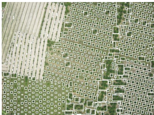
Figure 53 The result of detected oil palms from filtered image
