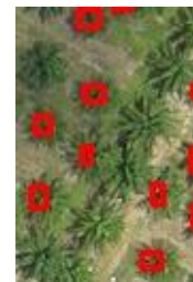
(b) The result of second erosion from Figure 73 (a) is on the left and the result of identification of individual oil palm is on the right
