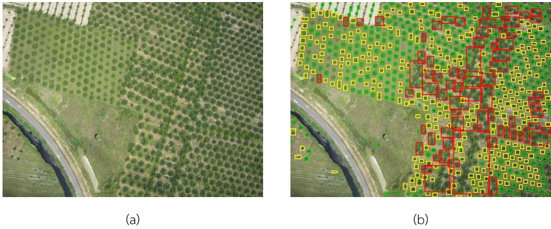
Figure 115 (a) original aerial image and (b) the result from applying K-means clustering
