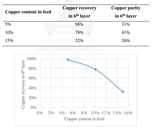
Figure 4. 12 Relationship between copper content in feed and copper recovery in the 6<sup>th</sup> layer
