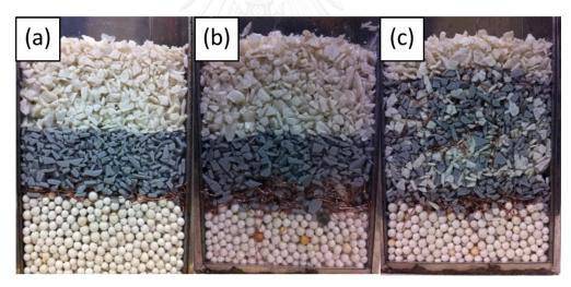
Figure 4. 10 Pictures of jig products of model samples with copper wires (30 mm long copper wires, separation time 3 minutes) at mass ratio variation; (a) 5 % (b) 10 % (c) 15 %
