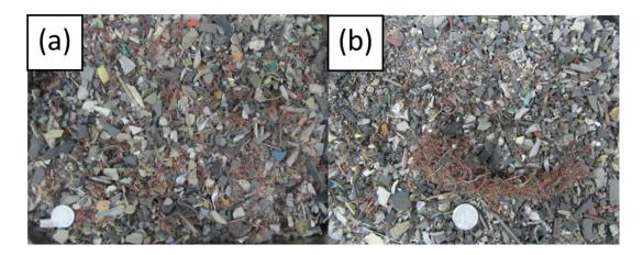
Figure 5. 6 Real sample; (a) before and (b) after pre-treatment by mill pot
