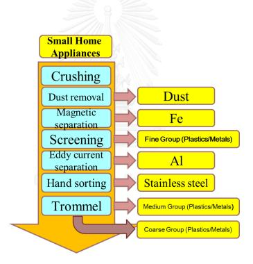
Figure 2. 15 Recycling flowchart of small home appliances of Re-Tem Corporation (Pilot scale)
