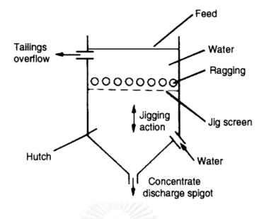
Figure 2. 5 Basic Jig Construction
