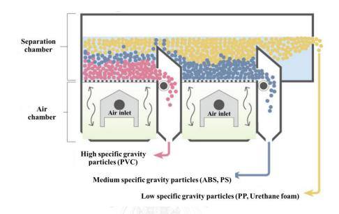
Figure 2. 12 Schematic outline of the continuous RETAC jig
