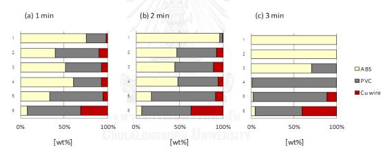
Figure 4. 9 Components of each layer after jig separation of model samples with copper wires (10 wt% copper wires, 30 mm long copper wires) at separation time variation; (a) 1 minute (b) 2 minutes (c) 3 minutes
