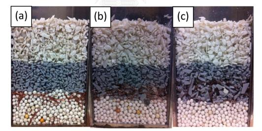
Figure 4. 13 Pictures of jig products of model samples with copper wires (10% copper wires, separation time 3 minutes) at lengths of copper wires variation; (a) 10 mm (b) 30 mm (c) 50 mm
