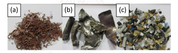
Figure 3. 2 Three fractions of real sample after hand sorting; (a) copper wires, (b) others metals, and (c) plastics & PCB
