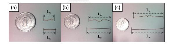
Figure 3. 13 Absolute maximum lengths of entangled copper wires:  $L_e$  and real length of straight copper wires:  $L_s$ ; (a) 10 mm (b) 30 mm (c) 50 mm
