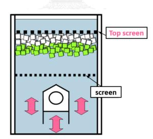
Figure 2. 9 Schematic outline of the desktop type batch-wise reverse jig
