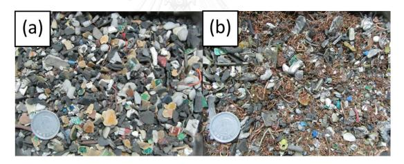
Figure 5. 10 Jig products of real sample (with pre-treatment); (a) 5<sup>th</sup> layer and (b) 6<sup>th</sup> layer
