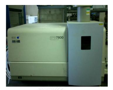
Figure A-3 Inductively Coupled Plasma-Atomic Emission Spectrometry (ICP-AES) (Seiko Instruments Inc., Ltd., SEIKO-SPS7800) at the Laboratory of Mineral Processing and Resources Recycling, Division of Sustainable Resources Engineering, Graduate School of Engineering, Hokkaido University, Japan
