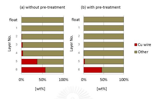
Figure 5. 9 Components of each layer after jig separation of real sample; (a) without and (b) with pre-treatment
