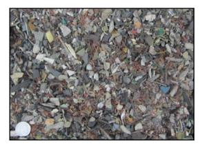
Figure 3. 1 Crushed end-of-life small home appliances sample (the fine fraction)
