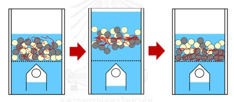
Figure 4. 16 Entanglement phenomena during jig separation (white circles: ABS, grey circles: PVC, and red line: copper wires)
