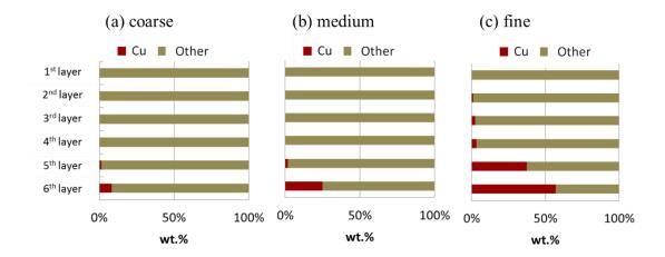
Figure 2. 19 Components of each layer after jig separation; (a) coarse group, (b) medium group, and (c) fine group
