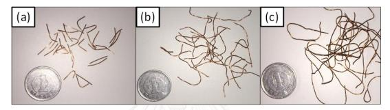
Figure 3. 12 Copper wires in the model samples; lengths (a) 10 mm, (b) 30 mm, and (c) 50 mm.
