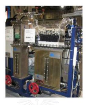
Figure 2. 13 Laboratory scale RETAC jig; batch (left) and continuous type (right)
