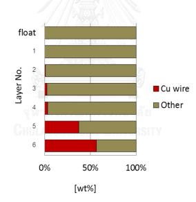
Figure 4. 3 Components of each layer after jig separation of real sample
