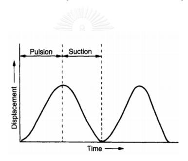
Figure 2. 3 Movement of the piston in a jig
