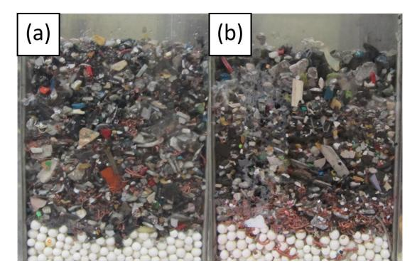
Figure 5. 8 Pictures of real sample (with pre-treatment) in separation chamber; (a) before and (b) after jig separation
