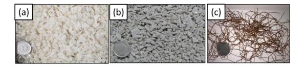
Figure 3. 9 Mixture of model samples; (a) ABS, (b) PVC, and (c) copper wires
