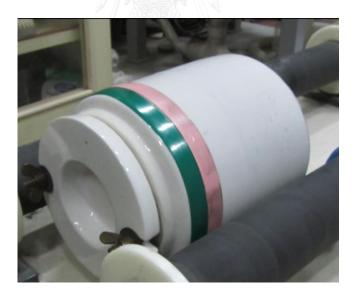
Figure 5. 1 Mill pot; inner diameter 190 mm
