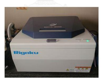
Figure A-2 X-ray fluorescence (XRF) Spectroscopy (Rigaku Corporation, Japan, Rigaku EDXL300) at the Laboratory of Mineral Processing and Resources
