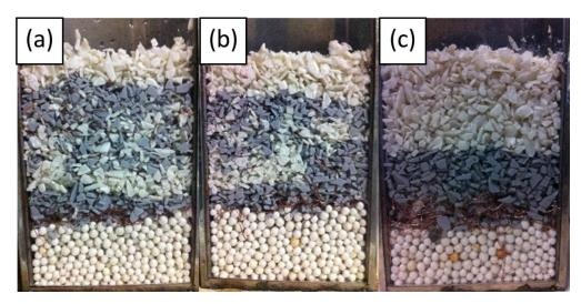
Figure 4. 8 Pictures of jig products of model samples with copper wires (10 % copper wires, 30 mm long copper wires) at separation time variation; (a) 1 minute (b) 2 minutes (c) 3 minutes
