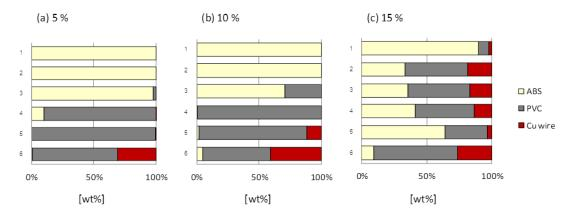
Figure 4. 11 Components of each layer after jig separation of model samples with copper wires (30 mm long copper wires, separation time 3 minutes) at mass ratio variation; (a) 5 % (b) 10 % (c) 15 %
