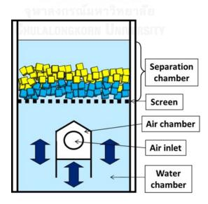
Figure 2. 7 Schematic outline of the desktop type batch-wise RETAC jig
