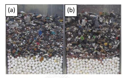
Figure 4. 2 Pictures of real sample in separation chamber; (a) before and (b) after jig separation
