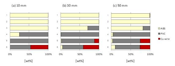
Figure 4. 14 Components of each layer after jig separation of model samples with copper wires (10 % copper wires, 3 minutes) ) at lengths of copper wires variation; (a)10 mm (b) 30 mm (c) 50 mm
