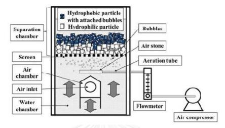
Figure 2. 10 Schematic outline of the desktop type batch-wise hybrid jig
