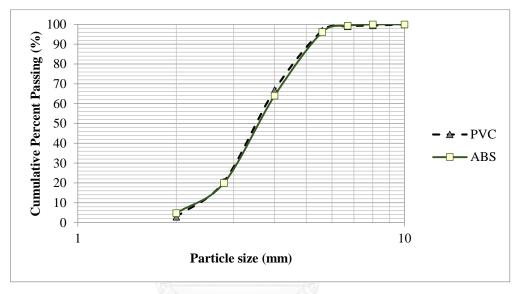
Figure 3. 11 Particle size distributions of the plastics mixture in model samples
