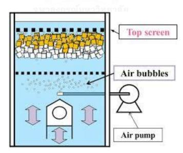
Figure 2. 11 Schematic outline of the desktop type batch-wise reverse hybrid jig
