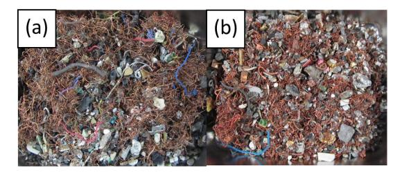
Figure 4. 4 Jig products of real sample; (a) the 5<sup>th</sup> layer and (b) the 6<sup>th</sup> layer
