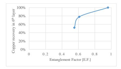
Figure 4. 15 Relationship between entanglement factor [E.F.] and copper recovery in the 6<sup>th</sup> layer
