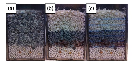
Figure 4. 5 Example pictures of model samples in separation chamber; (a) before jig separation, (b) after jig separation, and (c) upon divided into 6 layers
