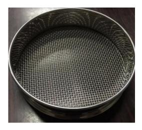
Figure 5. 2 Sieve; aperture size 16 mm.
