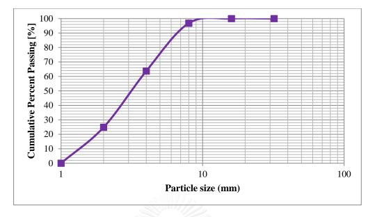
Figure 3. 6 Particle size distribution of the real sample
