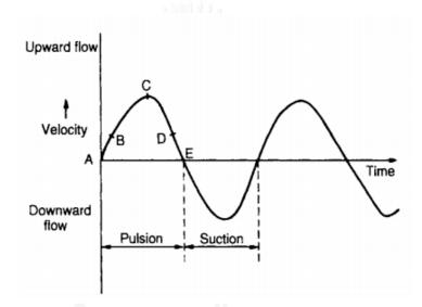
Figure 2. 4 Speed of flow through bed during jig cycle
