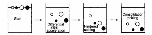
Figure 2. 2 Idealized jig separation process
