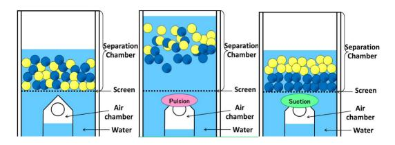
Figure 2. 8 Separation process of RETAC jig
