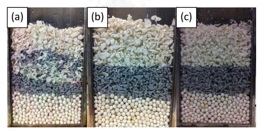
Figure 4. 6 Picture of jig product of model sample (without copper wire) at separation time variation; (a) 1 minute (b) 2 minutes (c) 3 minutes
