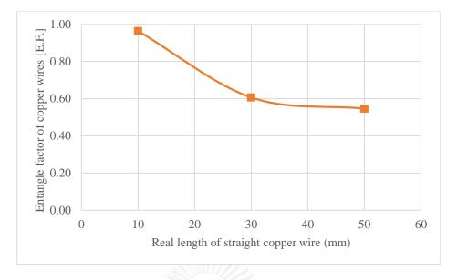
Figure 3. 14 Relationship between Entangle factor of copper wires [E.F.] and Real length of straight copper wire (mm)
