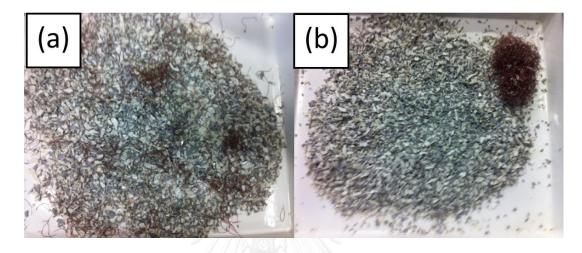
Figure 5. 4 Model sample; (a) before and (b) after pre-treatment by mill pot
