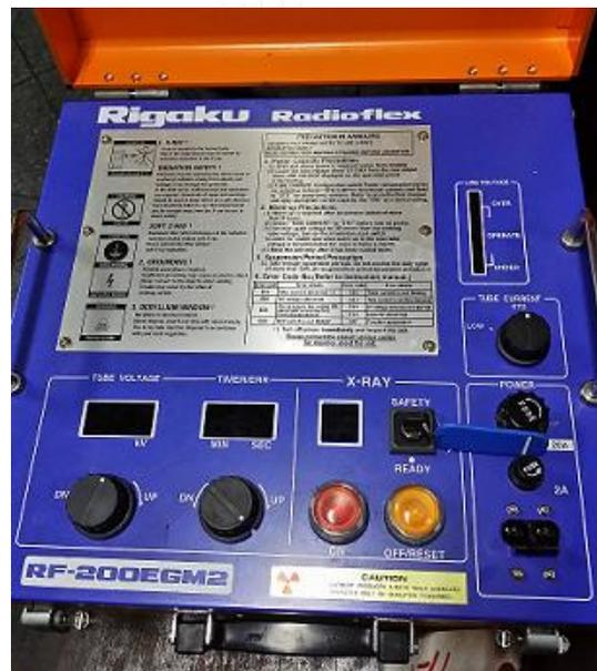
Figure 3.2 Control panel of the Rigaku Radioflex RF200EGM2 X-ray Machine
