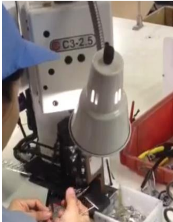
Figure 4-15 Crimping terminal of G/Y and R/L wire
