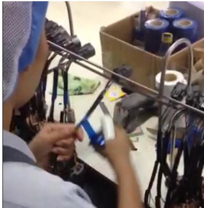
Figure 4-17 Taping top part of cable
