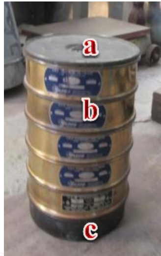
Figure 2.7 Nest: a. Lid, b. Sieve, c. Pan (Mining Laboratory at Chulalongkorn University, 2015)
