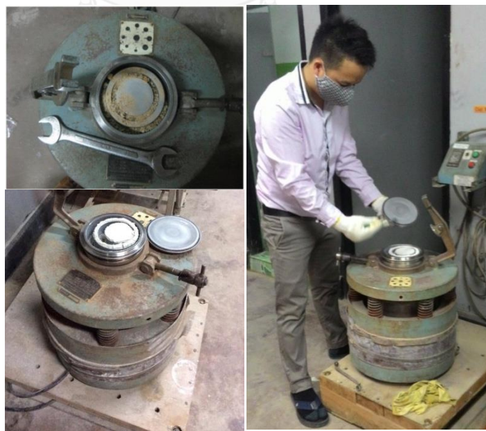
Figure 3.8 Vibratory cup mills
