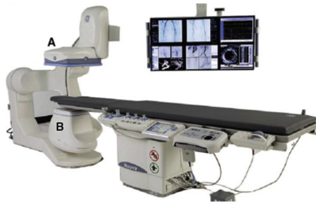
Figure 2. 9 Photograph shows a large FPD fluoroscopy system. A- Flat-panel image receptor. B- X-ray tube.
