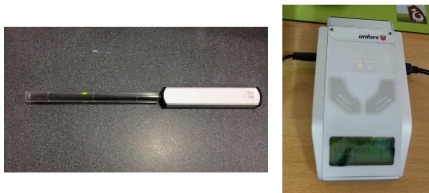
Figure 3. 6 Unfors Xi CT Detector 10 cm length of the pencil-type ionization.
