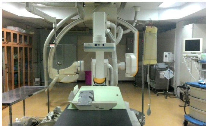
Figure 3. 2 DSA Biplane Flat panel detector Siemens Axiom Artis.
