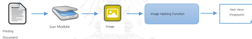
Figure 2. Fingerprint capturing process of printing document via image hashing function
