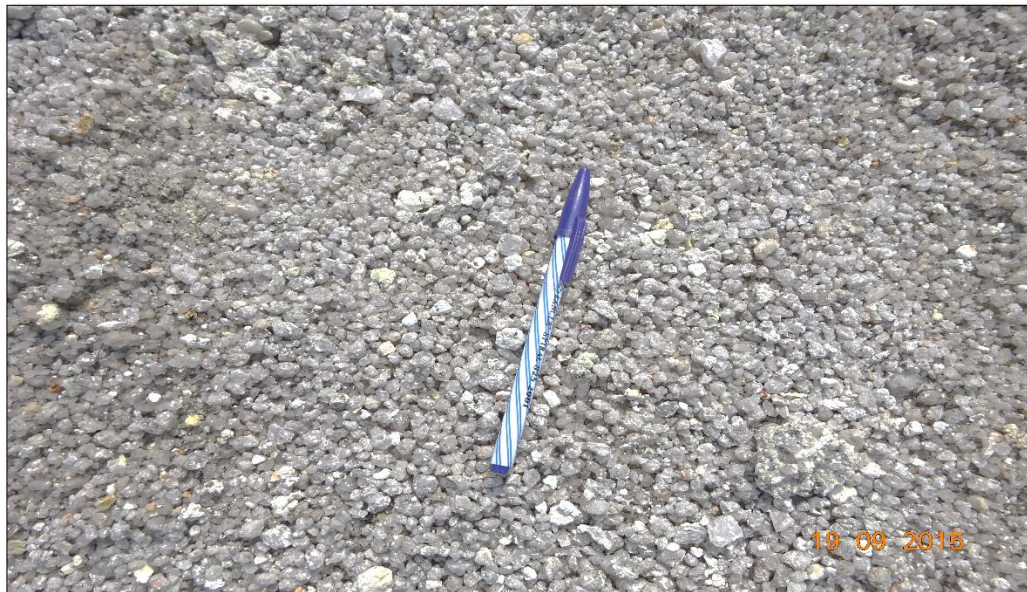
Figure 4. 4 Coarse-grained size of quartz in kaolin mine, photo at the floor of Pit MF-10
