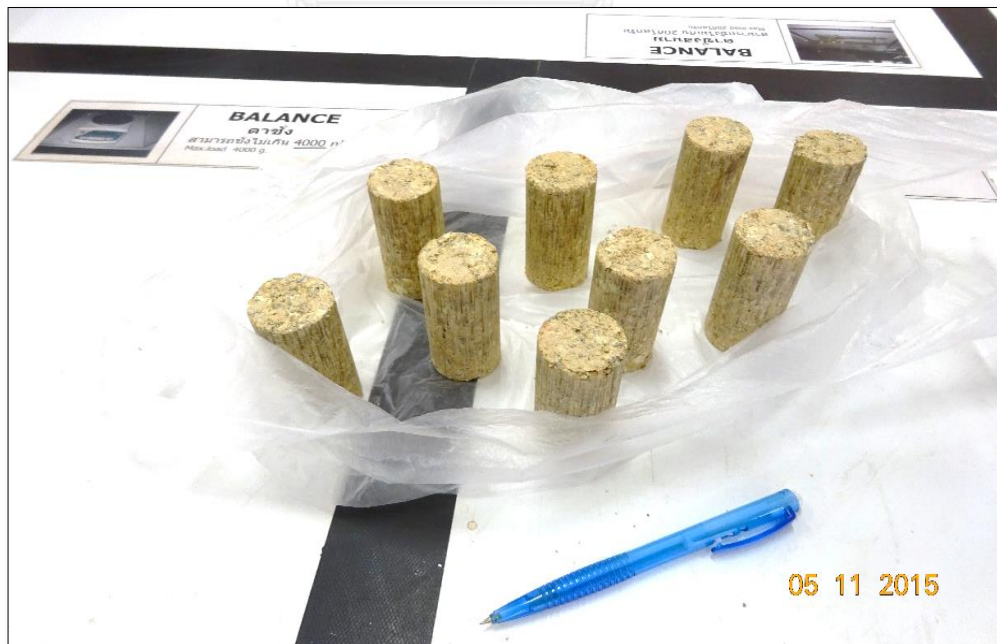
Figure 3. 8 Remolded specimens used in unconfined compression and UU triaxial test.
