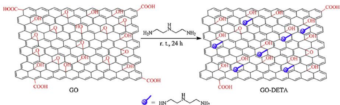
Figure 2.8 Structure of surface modified GO (Yang, Li et al. 2015)
