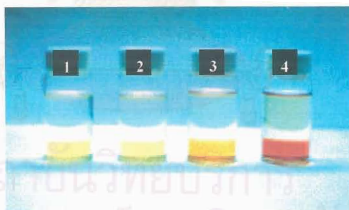
Figure 4-8 Color of extract phase (lower phase) of azo dyes from CNSL hexyl ester coupling with
