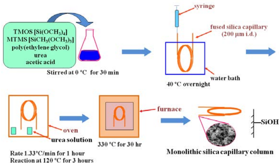
Figure 3.2 The diagram for preparation of monolithic silica capillary column
