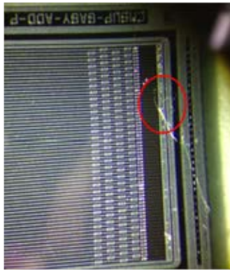
Figure 4.16: Scratch on the bias resistors and the bias ring of F200DP_05_Badd_1 sensor resulted in broken bias resistors, high leakage current on the broken strip (strip no.44-54), and high total leakage current ( 25 \mu\text{A} @200V 20°C).
