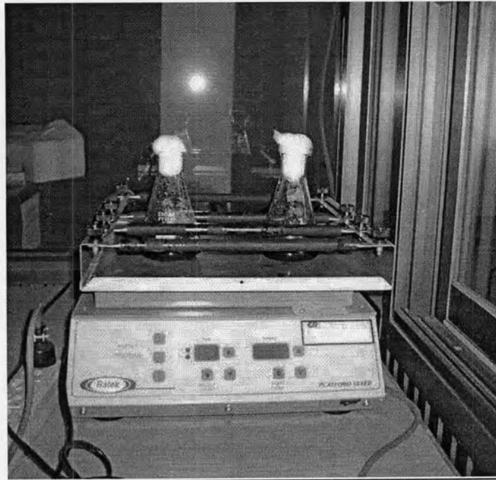
Figure 3-4 Inoculation of Biofilter Media in Liquid Medium
