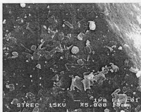
Figure 4.6 SEM micrograph of AHAMAA prepared with 4 \times 10^{-3} mol AA, 2.3 \times 10^{-4} mol N-MBA, 1.6 \times 10^{-4} mol APS and 12 \times 10^{-4} mol TEMED
