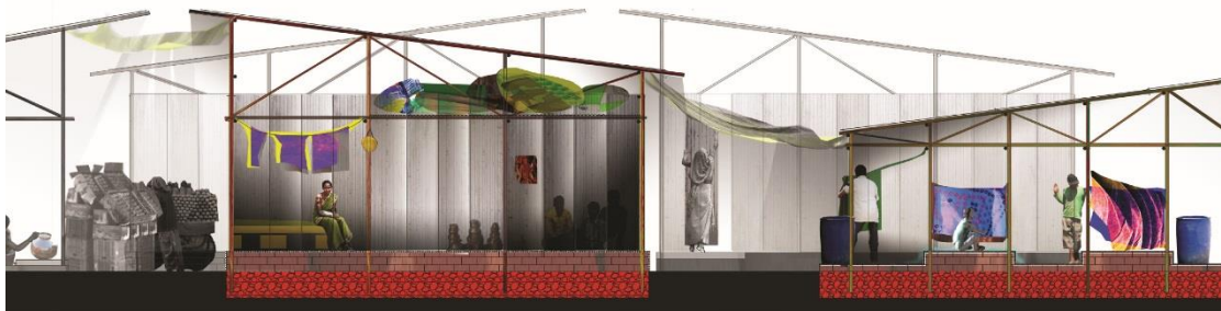
Figure 38. Section of the design concept presenting the shadings and double roofs
