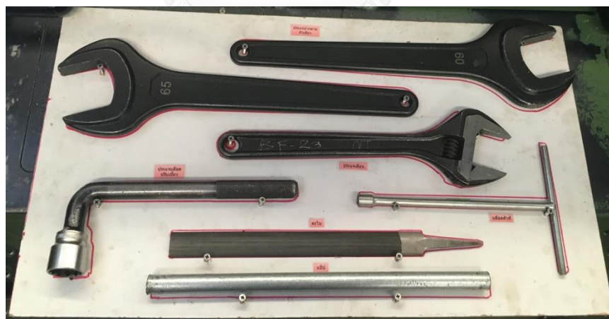
Figure 66: shadow board for bolt forming setup operation
