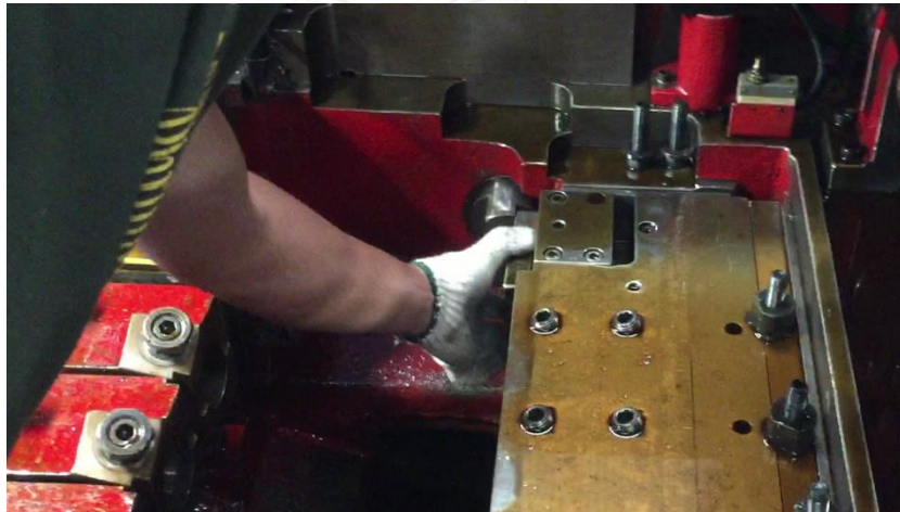
Figure 82: Step 7A Mount new wire toolings onto machine
