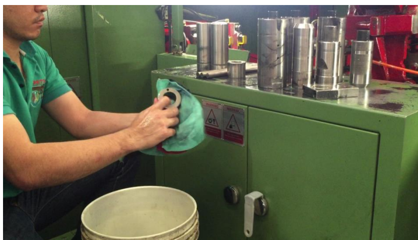
Figure 34: Step 10 Clean up the previous dies, punches and wire toolings
