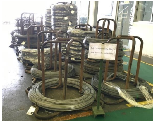
Figure 16: Steel wire rod (finished wire) as raw material for bolt forming process
