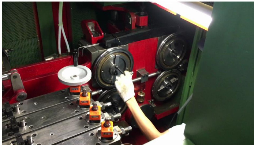
Figure 33: Step 9 Dismount the previous feeding rollers
