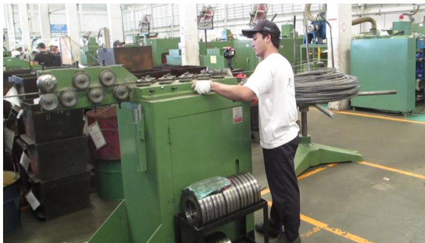
Figure 94: Step 5B Connect finished wire onto machine
