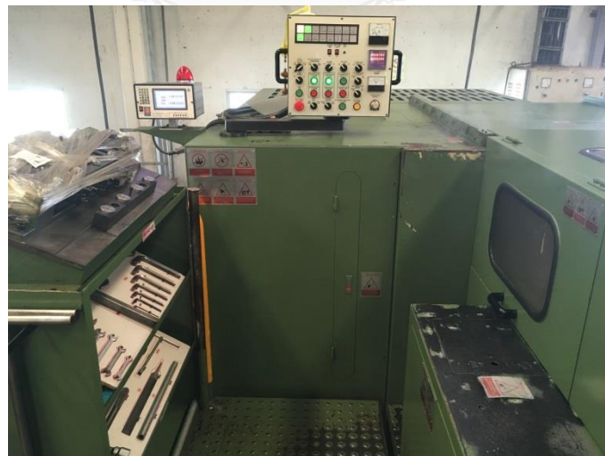
Figure 68: Setup operation area on bolt former
