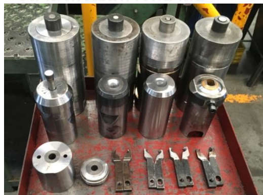
Figure 17: Toolings for bolt forming setup operation
