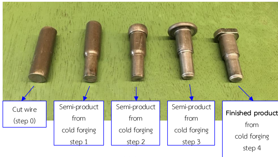
Figure 19: Example of four step transformation product
