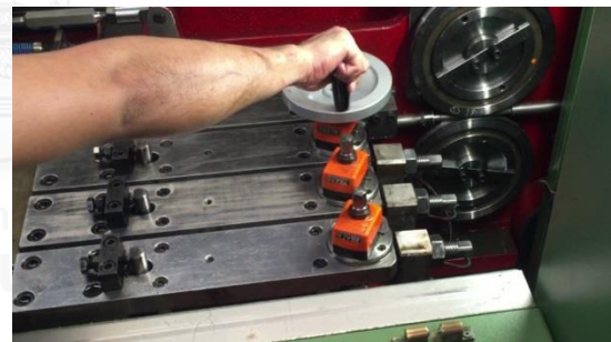
iii) Make adjustment on punch side (left) and die side (right)
