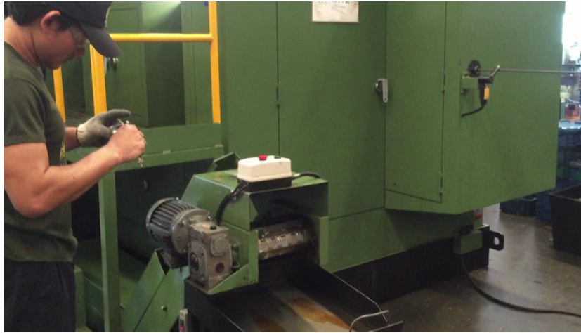
Figure 87: Step 11A Test run machine at production speed
