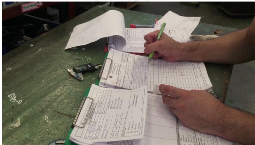
Figure 42: Step 18 Fill in First Piece Inspection Check Sheet
