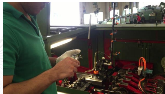
ii) Pick up product from gripper and check sizes of product using measuring tools
