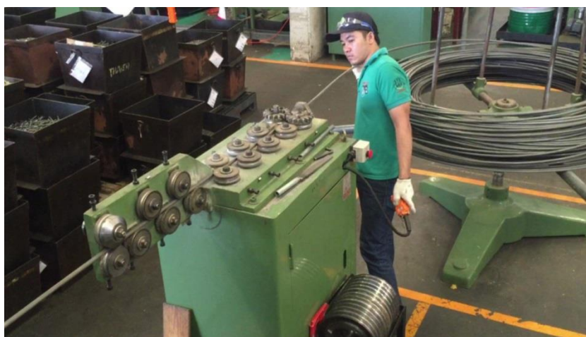
Figure 37: Step 13 Connect finished wire onto machine
