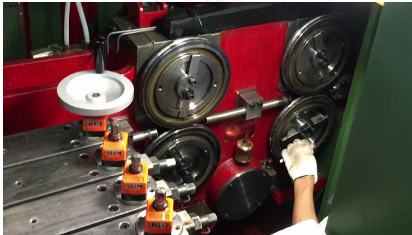
Figure 36: Step 12 Mount new feeding rollers onto machine
