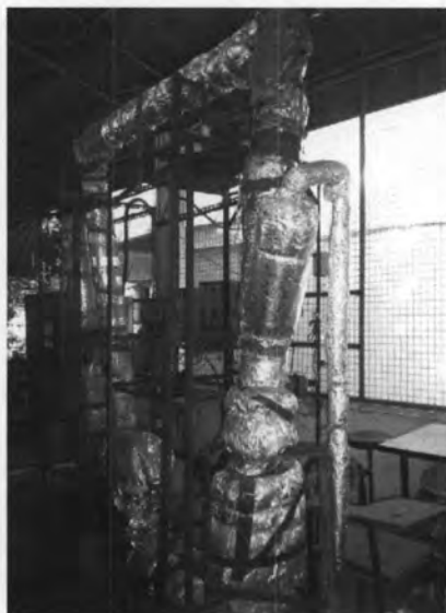
Figure 2.8 A batch hot air fluidized bed dryer
