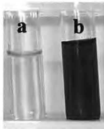
Figure 3.1 Appearance of PCDA hydrocolloid irradiated with UV light after a) stored at room temperature and b) stored in a refrigerator overnight.
