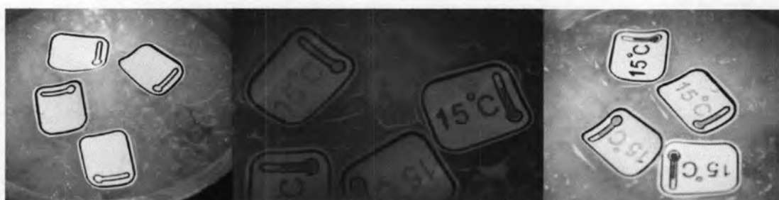
Figure 3.51 Polymerization of temperature indicating MPCDA screen ink in an ice bath.
