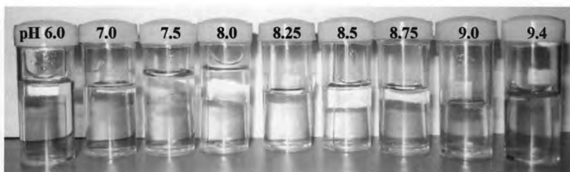
Figure 3.22 Color photographs of 12-layered chitosan/poly(PCDA) films in various pH phosphate buffer (100 mM).
