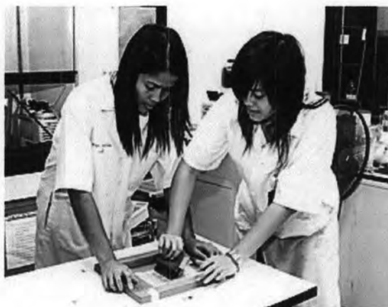
Figure 3.49 Screening of temperature indicating screen ink
