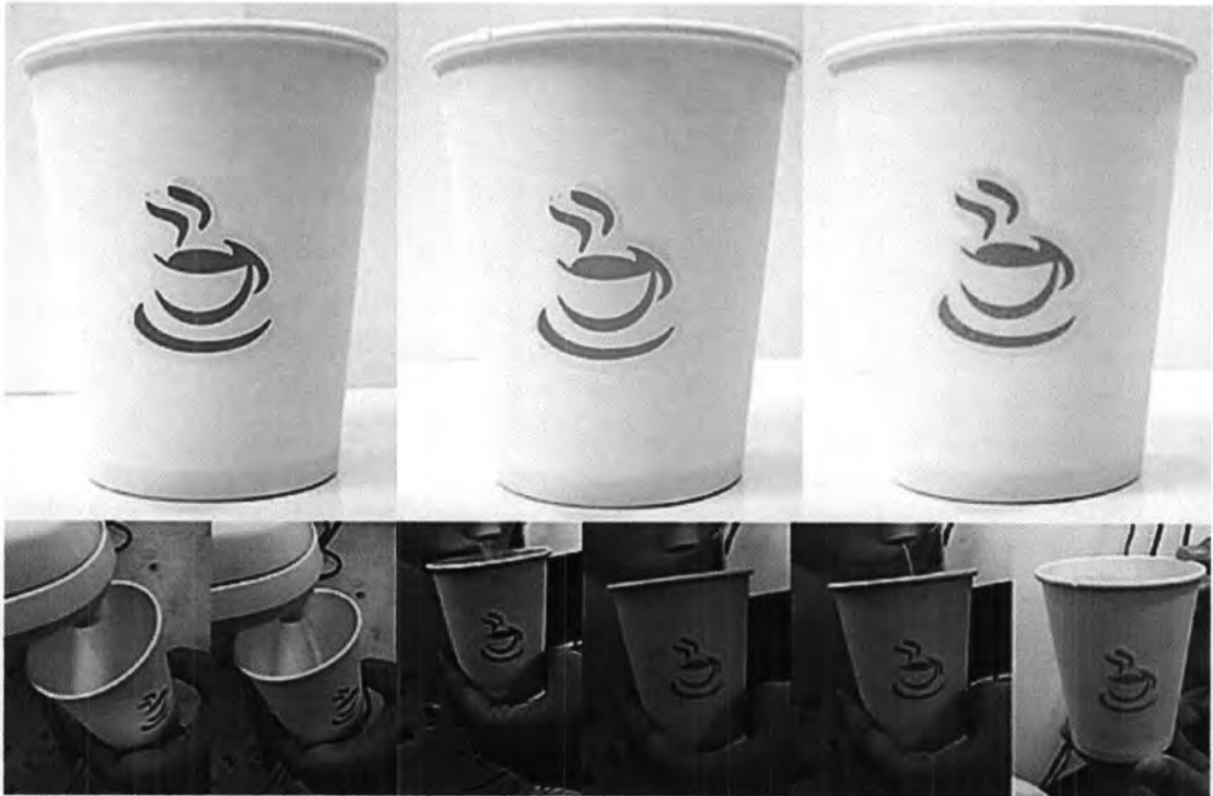
Figure 3.53 Using of temperature indicating label with hot cup. (left) PCDA label before given heat, (middle) PCDA label after given heat, (right) EBPCDA label, (below) Color changing of PCDA label during addition hot water.
