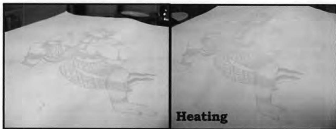
Figure 3.43 Graphic images, produced by 5 times reprinting from an inkjet printer using 1 mM poly(EBPCDA) sol as an ink, before and after heating with a hair blower.
