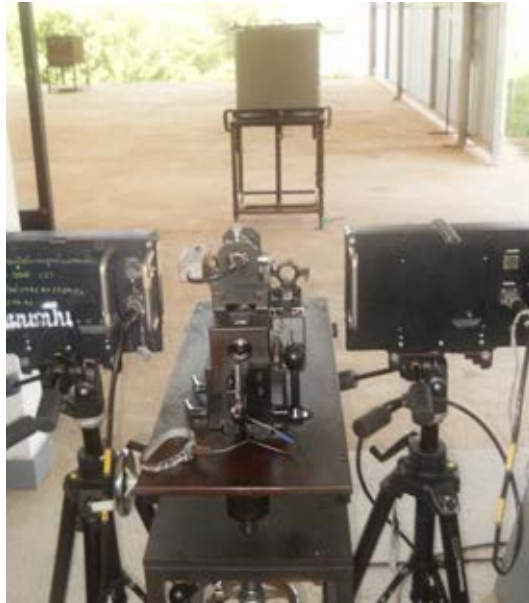
(a.) Equipments set up following NIJ standard level III
