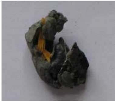
The deformed bullet retrieved from 1 panel of glass fiber composite
