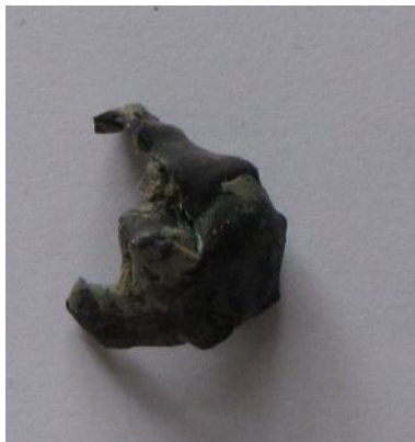
The deformed bullet retrieved from 2 panels of glass fiber composite
