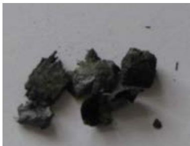
The deformed bullet retrieved from 1 panel of carbon fiber composite
