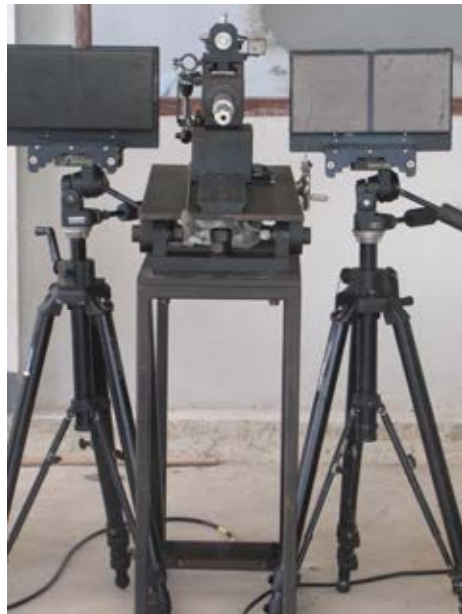
(b.) Test barrel and chronographs
