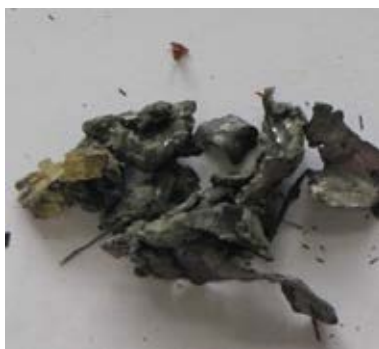
The deformed bullet retrieved from 2 panels of carbon fiber composite
