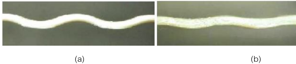
Figure 2.10 (a) Crimp in warp and (b) weft yarns from Twaron™ CT716 fabric.
