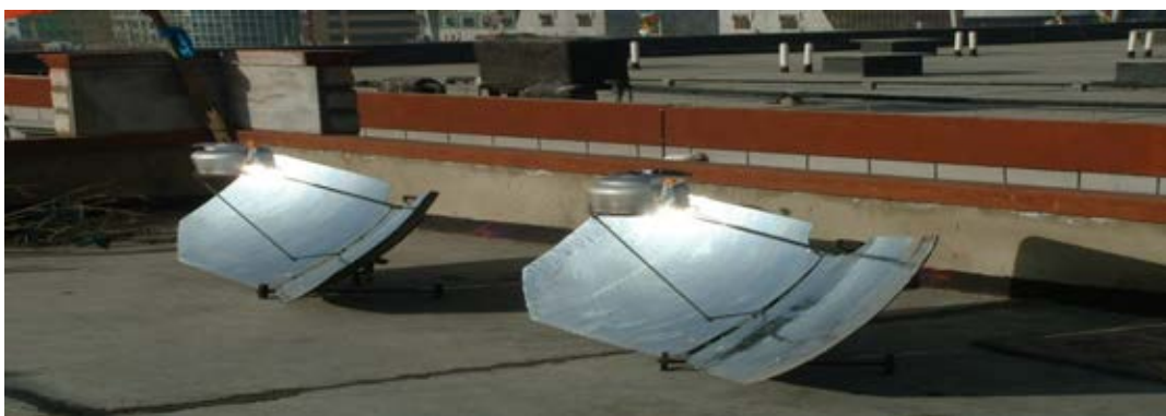
Picture 6.1: Sample of Solar Cooking Technology(Professor Toh Peng Seng's Photograph)
