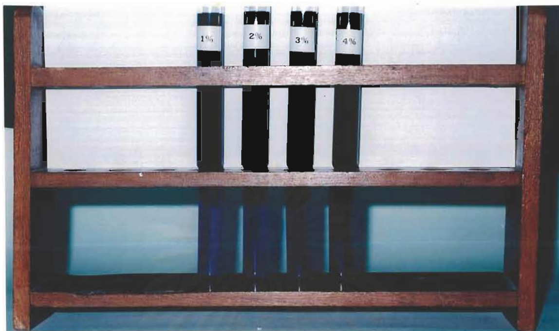
Figure 4.18 The comparison between the color of dye bath solution before (top) and after (below) dyeing of synthesized cationic reactive dye.
