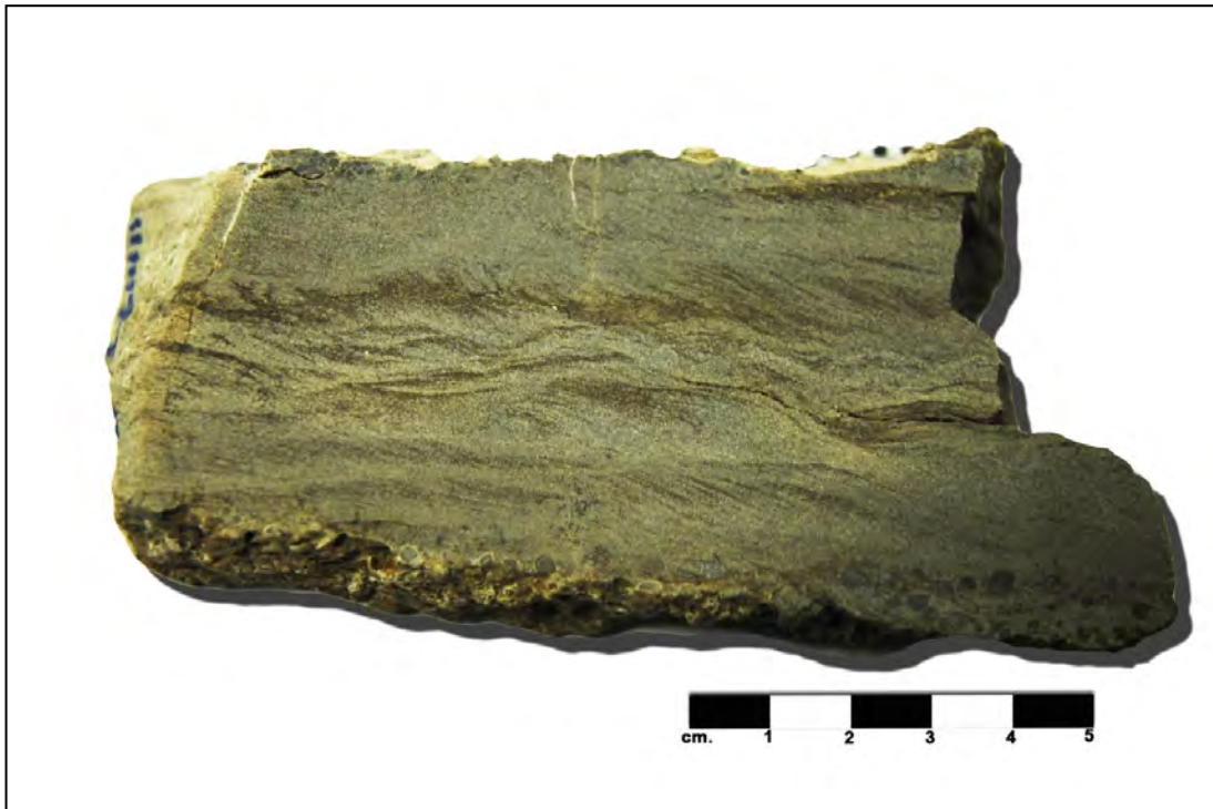
Fig 2.17 Fined-grained sandstone shows cross-bedding in lower and upper, and wavy structure in middle.
