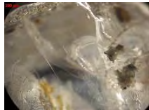
Fig.A8 Needle inclusions and fingerprints (sample C8)
