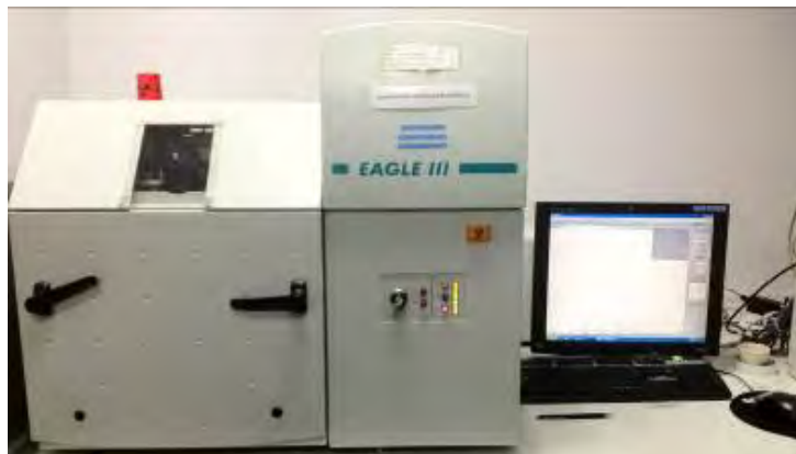
Fig. 2.11 Energy Dispersive X-Ray Fluorescence Spectrometer (model EAGLE III) at GIT.
