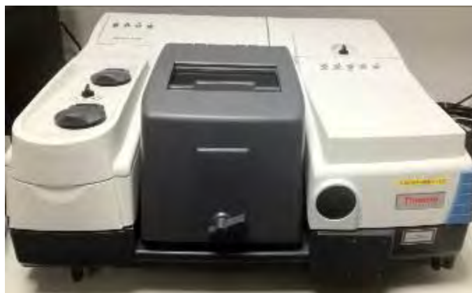
Fig. 2.8 Fourier Transform Infrared Spectrophotometer (NICOLET 6700) at GIT
