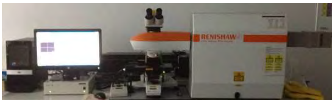
Fig. 2.7 Laser Raman Spectroscopy (Model 1000, Renishaw) at GIT
