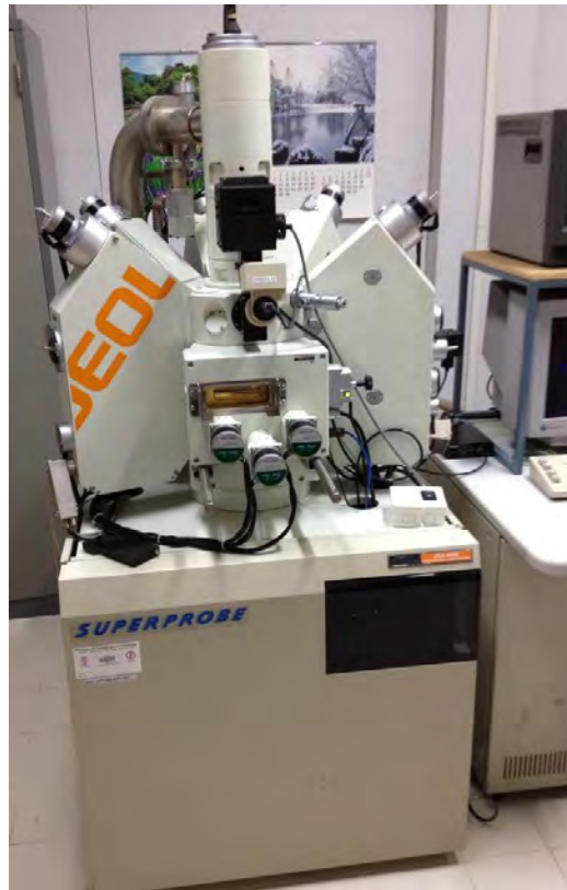
Fig. 2.10 Electron Probe Micro-Analyzer (JEOL JXA-8100) based at Geology Department, Faculty of Science, Chulalongkorn University
