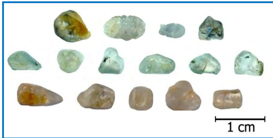
Fig.4.1 Group 1 samples of Deniyaya sapphires for heating at 1,650°C in reducing atmosphere.
