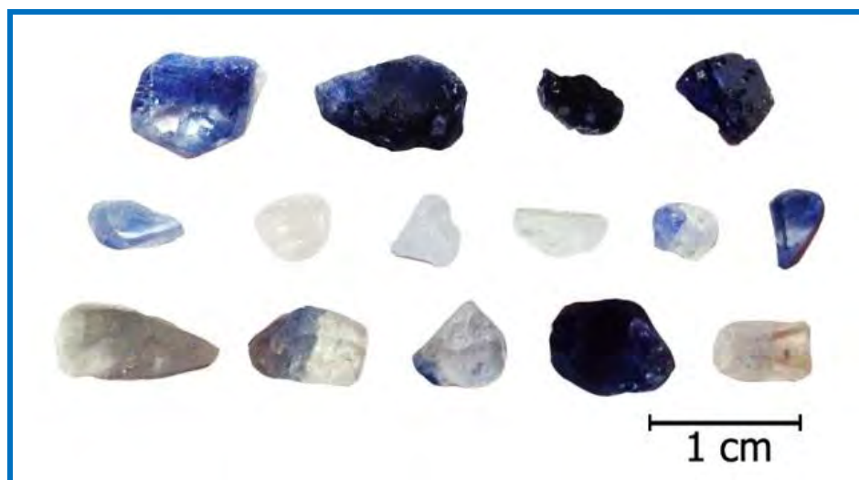
Fig.4.3 Color changing of Group1 Deniyaya sapphires after heat treatment in reducing atmosphere.
