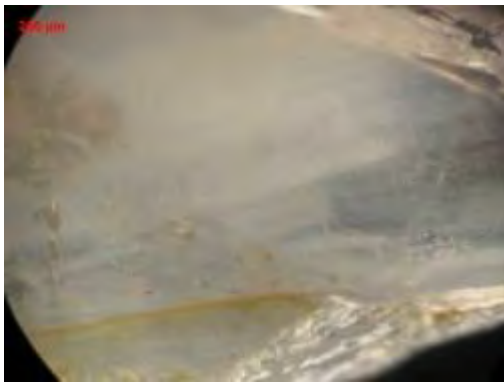
Fig.A3 Cloud and small rutiles (sample C1)
