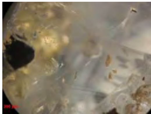
Fig.A12 Fingerprints, rutiles and fractures (sample Y8)
