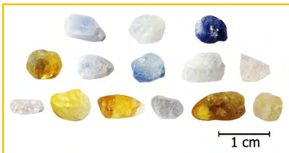
Fig.4.3 Color changing of Group1 Deniyaya sapphires after heat treatment in reducing atmosphere.
