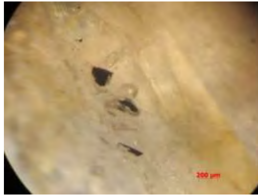
Fig.A10 Negative crystals and cloud (sample Y4)
