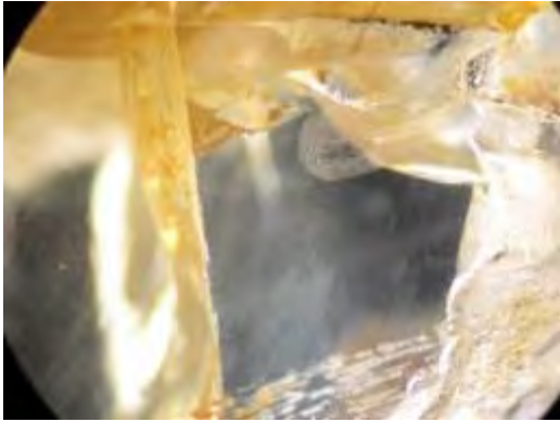
Fig.A1 Fingerprints and cloud (sample B1)
