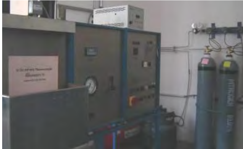
Fig. 2.13 Linn electric furnace, Model HT 1800 Plus VAC Bottom Loader at Department of Geology, Faculty of Science, Chulalongkorn University.
