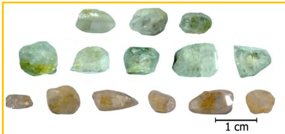
Fig.4.2 Group 2 samples of Deniyaya sapphires for heating at 1,650°C in oxidizing atmosphere.
