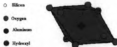
Figure 2.3 Aluminum octahedron, \text{Al}(\text{OH})_6^{3-} [18].
