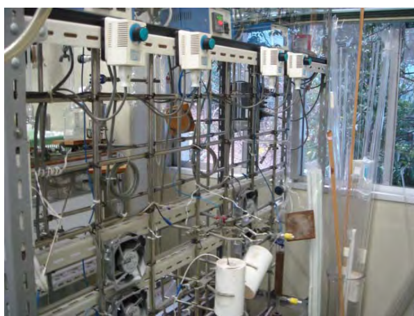
Figure 3.54 Heating machine for remove Oxygen gas
