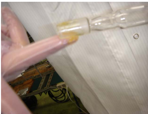
Figure 3.45 Using grease around area bottom of tube
