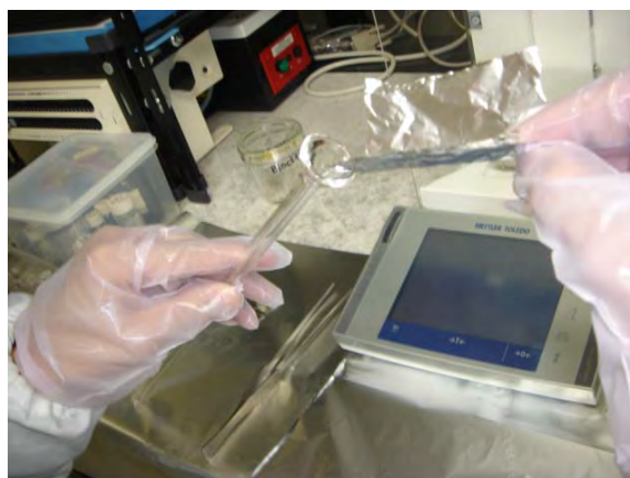
Figure 3.39 Put both of Copper Oxide and Plant sample into tube together
