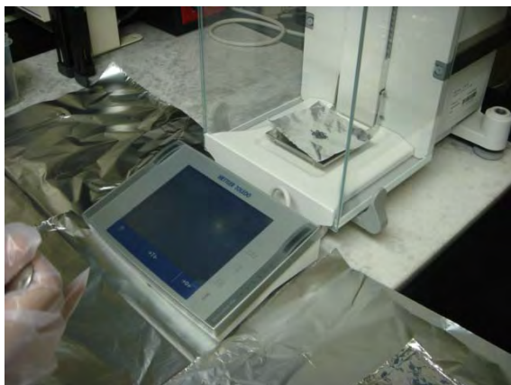
Figure 3.32 Weigh Copper Oxide around 500 mg.
