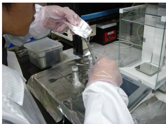
Figure 3.33 Put Copper Oxide and Oxalic acid into tube together
