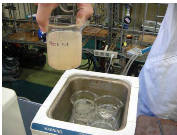
Figure 3.22 Change distilled water until distilled water did not change color (around 5 times)
