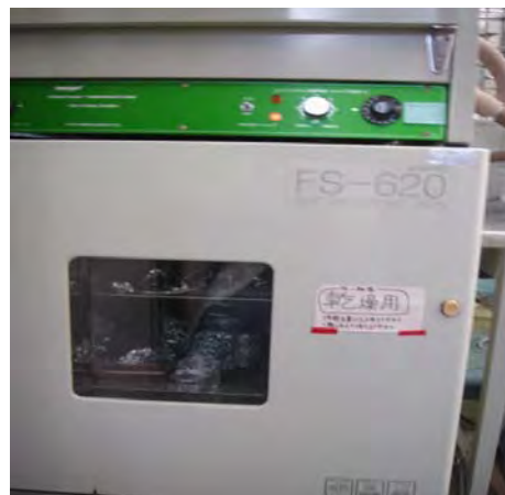
Figure 3.25 Bring shells samples into Electric drying oven wait 1-2 hours
