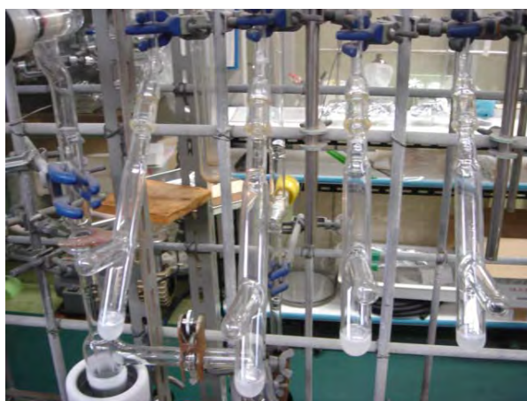
Figure 3.46 Connect tubes into evacuated grass line
