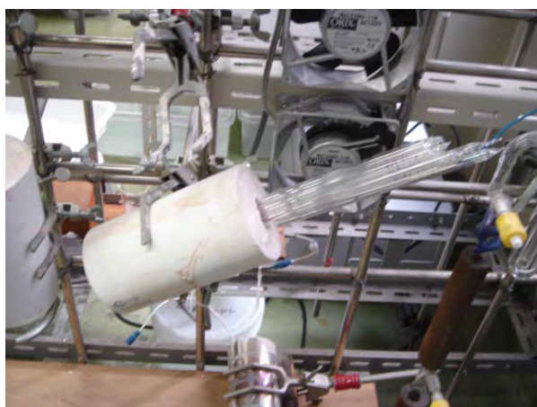
Figure 3.58 After cutting bring tube to heat with temperature 650° c wait 6 hours
