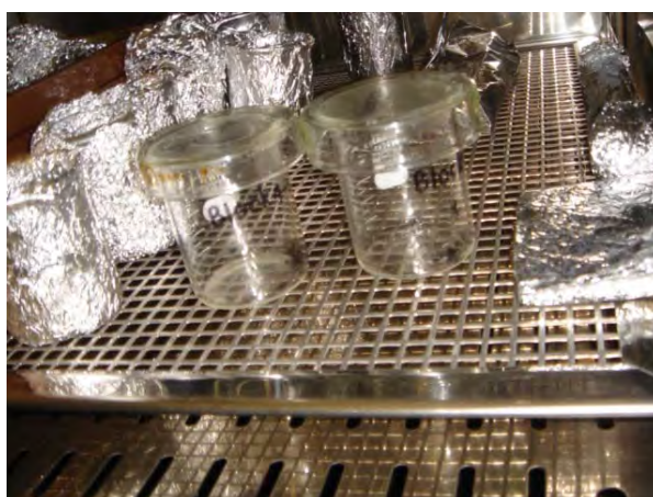
Figure 3.31 Bring them into Electric drying oven temperature 90° c wait 3 hours.
