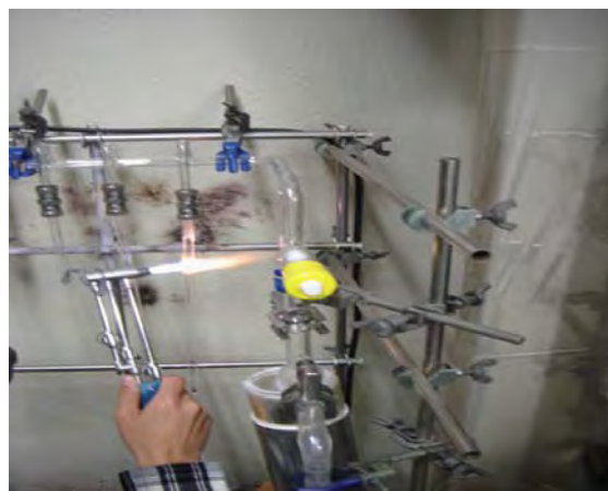
Figure 3.41 After wait 3 hours cut tubes and bring tube into heater machine
