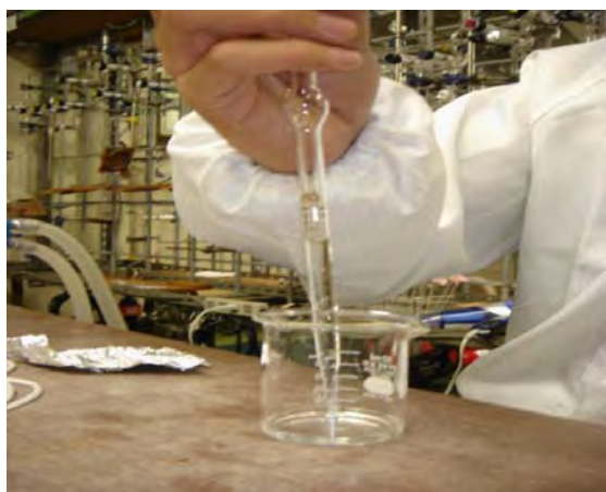
Figure 3.44 Use pipette for move Phosphoric acid 2 ml. and put it into tube
