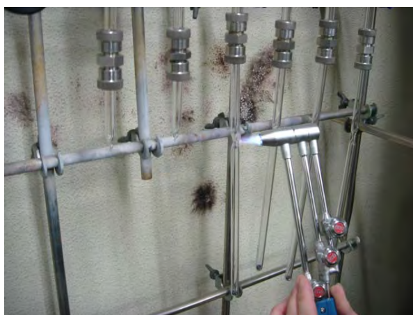
Figure 3.35 Cutting by fire
