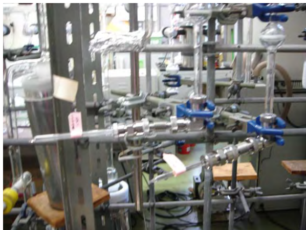
Figure 3.56 Connect sample tube into graphitization grass line
