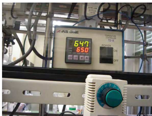
Figure 3.58 After cutting bring tube to heat with temperature 650° c wait 6 hours
