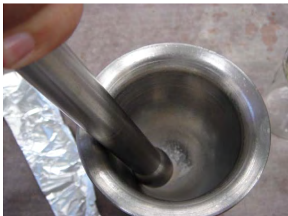
Figure 3.42 Broke shells samples by mortar until particle is fine grains
