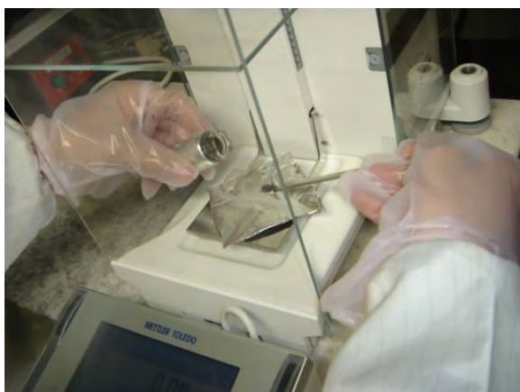
Figure 3.38 Weigh Copper Oxide
