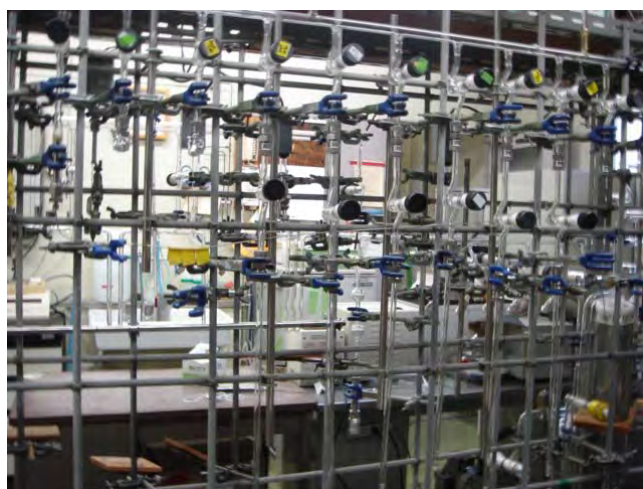
Figure 3.52 Connect tubes that has Iron powder into Hydrogen gas line
