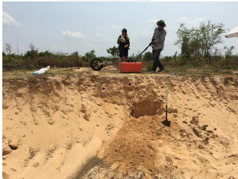
Figure 19 Survey line 8 from site no.2 of Mun River western part of Changwat Buriram. The site no.2 located on a point bar. This survey lite processes on the road cut profile by using GPR with 200 MHz antenna and documented a profile along with the survey.
