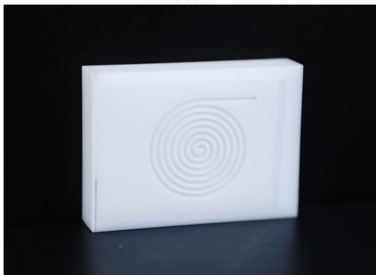
Figure 3.3 Chemiluminescence flow-cell with a spiral channel configuration.
