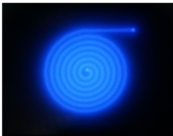
Figure 4.1 Chemiluminescence from the reaction of luminol with \text{H}_2\text{O}_2 and \text{K}_3\text{Fe}(\text{CN})_6 in a spiral flow-cell.
