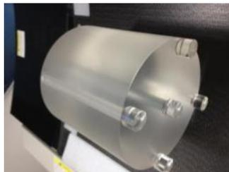
**Figure 3. 3** Cylindrical PMMA phantom of 16 cm diameter.
