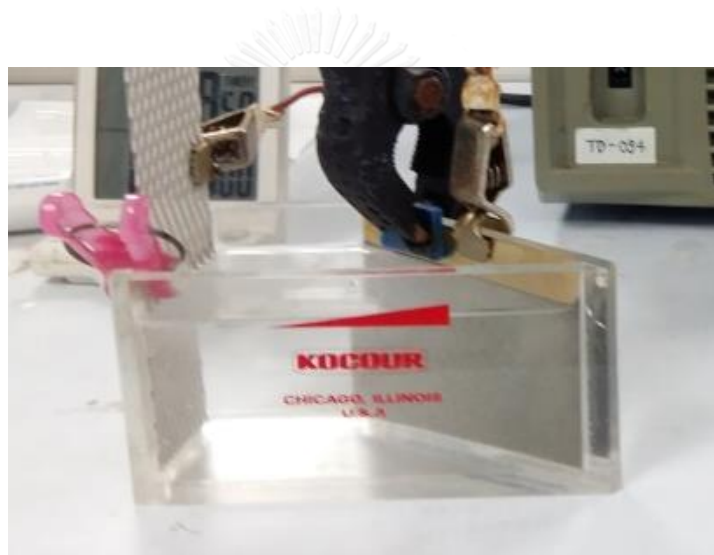
Figure 6 Hull Cell setup
