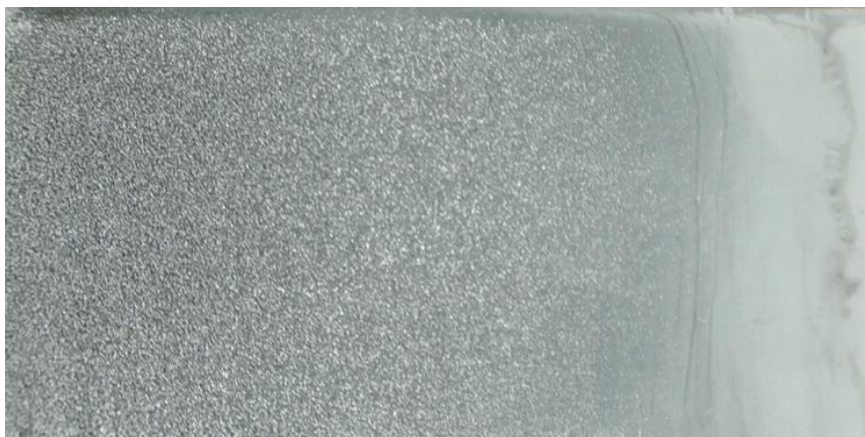
Figure 11 Hull cell test of zincate bath without additives.
