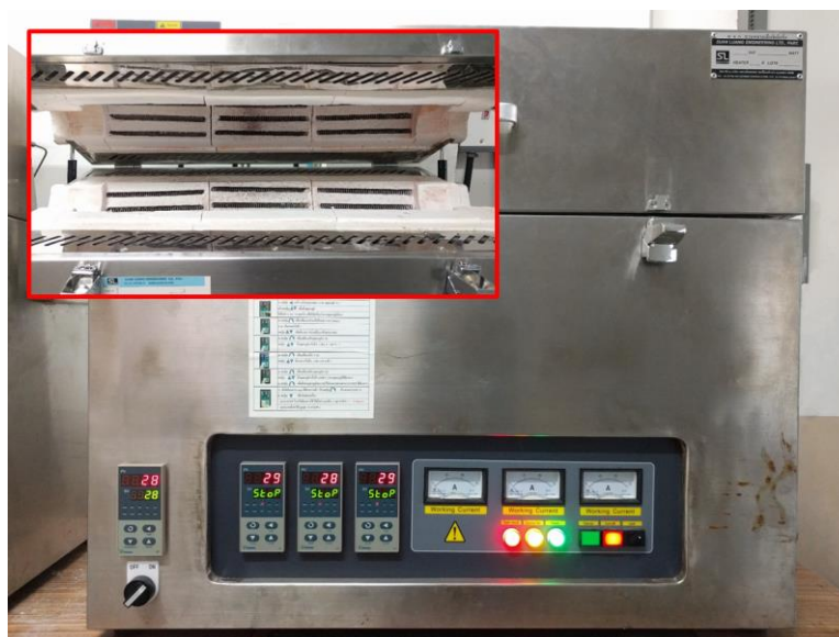
Figure 3.2 An electric furnace with temperature control
