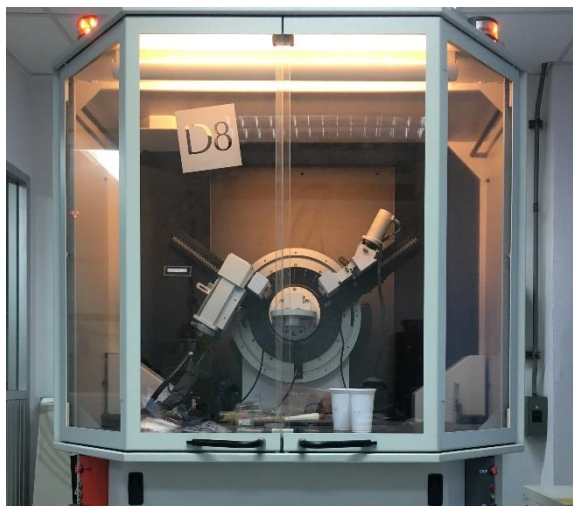
Figure 3.17 XRD; Bruker, D8 Discover
