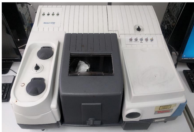
Figure 3.14 FT-IR; Thermo Scientific, Nicolet 6700
