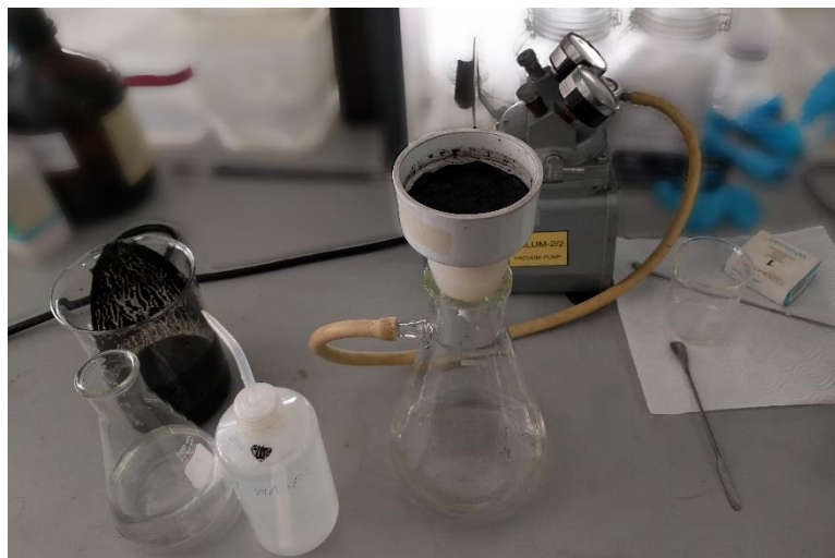
Figure 3.9 An apparatus for filtration of graphene oxide
