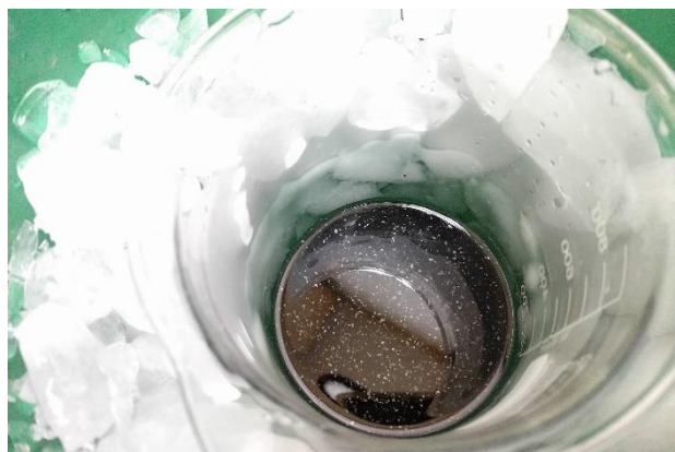
Figure 3.5 The mixture of graphite flake, sodium nitrate and sulfuric acid
