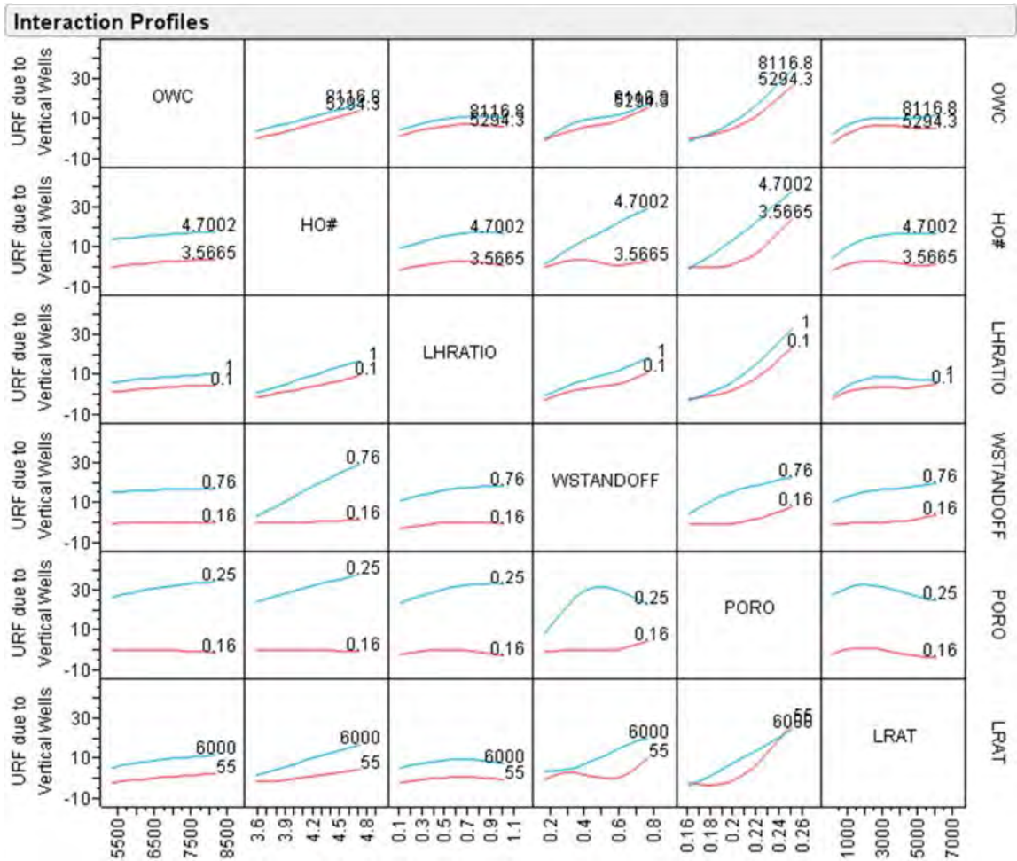
Figure E5: JMP interaction profiles at the optimum factor setting of the Gaussian process proxy model for vertical well production
