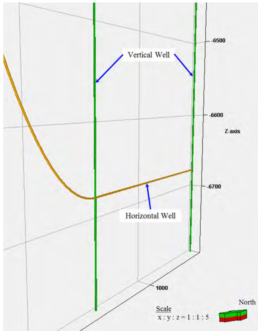
Figure 4.4: Locations of two vertical wells relative to a corresponding horizontal well
