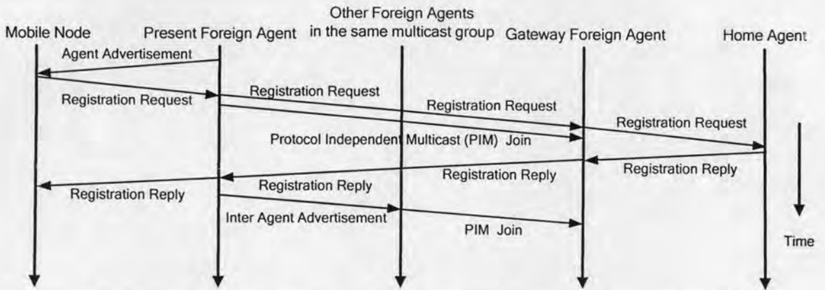
Figure 3.2 Signaling time diagram of initial registration in the proposed method.
