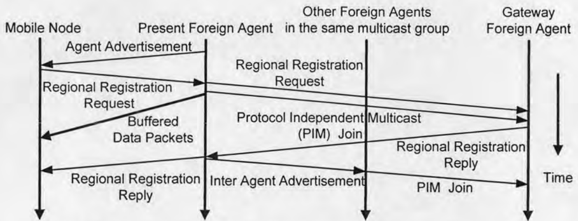
Figure 3.3 Signaling time diagram of regional registration process of an active Mobile Node in the proposed method.
