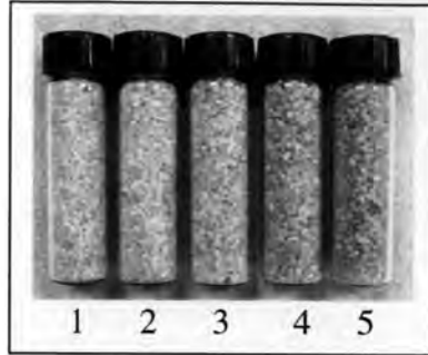
Figure 4.24 Comparison of carrier under different \text{Fe}^{2+} dosage. (*REMARK: 1. Original Carriers, 2. \text{Fe}^{2+} = 20 \text{ mg/l} , 3. \text{Fe}^{2+} = 50 \text{ mg/l} , 4. \text{Fe}^{2+} = 75 \text{ mg/l} , 5. \text{Fe}^{2+} = 100 \text{ mg/l} ).
