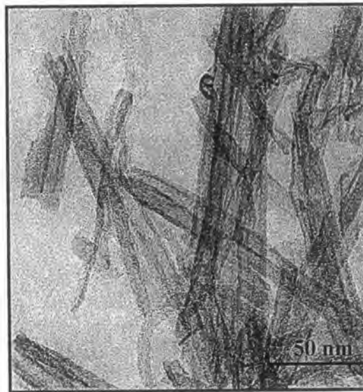
Figure 4.14 TEM image of TrCNT-TNT composite.
