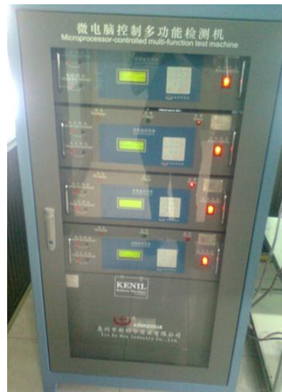
Figure 3.6 Battery charge/discharge and data processing control system (Xin Ke Hua Industry Co., Ltd)
