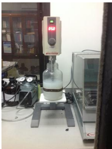
Figure 3.2 The setting of instrument for the gelled electrolyte preparation
