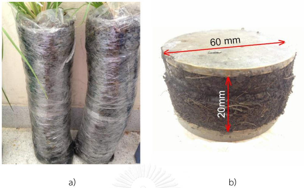
Figure 3-11: Single vetiver grass planting sample: a) before testing and b) after testing
