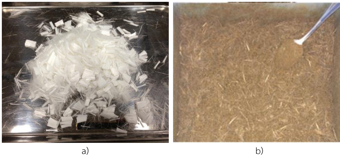
Figure 4-7: Polyester fibers before and after mixed with Edosaki sand at 2% by mass: a) Before mixing and b) After mixing
