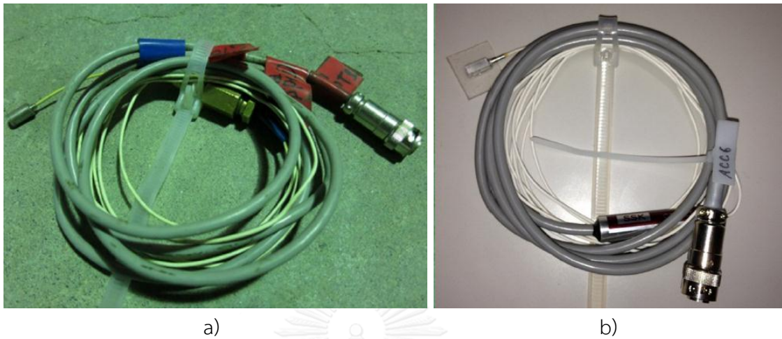
Figure 4-3: a) pore water pressure transducer and b) accelerometer
