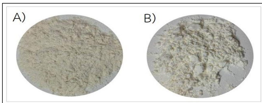
Figure 4.3 Powders of green mussel shells (A) before and (B) after treated with 0.5 M HCl solution.
