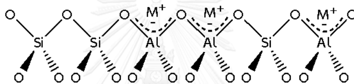
Figure 2.1 The general framework structure of zeolites
