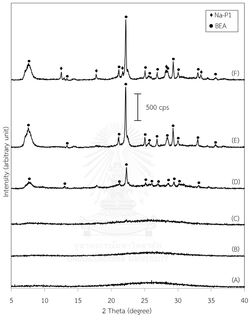
Figure 4.30 XRD patterns of as-synthesized zeolite beta products crystallized at 130 °C with various periods of crystallization: (A) 1 day; (B) 2 days; (C) 3 days; (D) 4 days; (E) 5 days and (F) 6 days
