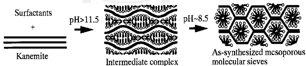
Scheme 2.1 Schematic models representing "folding sheets" mechanism
