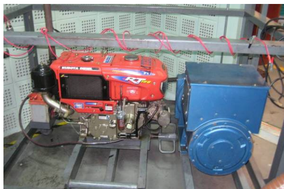
Figure 3.3 Single Cylinder Diesel Engine Connected with Generator
