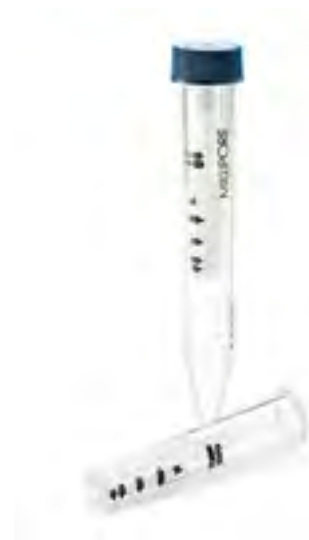
Figure 3.1 Centrifuge tube containing membrane with a cut-off molecular weight of 100,000 g/mol
