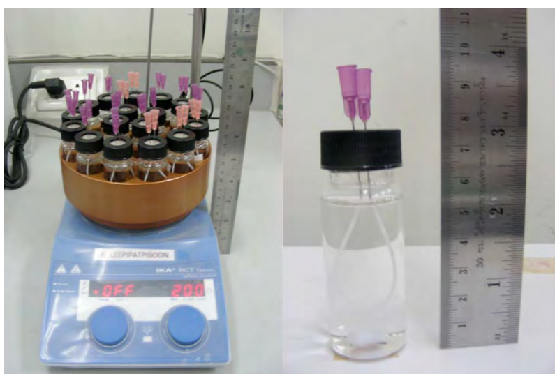
Figure 3.1 LPME device and multi-station magnetic stirrer
